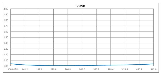
Click the following link (or enter part number in "SEARCH" on website) to obtain additional part information including price, inventory and certifications: Type N M/F Coaxial RF Surge Protector, 100MHz - 512MHz, DC Block, 750W, IP67, .5uJ, 20kA, Filter, Bracket Down, Hole Mount VHF50HN-MA
